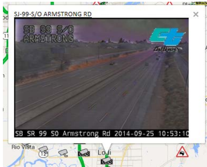
Figure 11: Caltrans D10 Image with Color Problem
