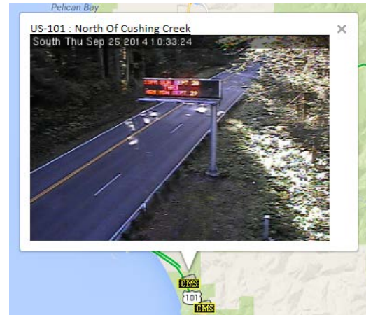
Figure 4: Caltrans District 1 CCTV Image to Confirm CMS Message
