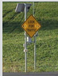
(Above) A rural intersection crash avoidance system in Wisconsin (Far left and below) The systems provide drivers (on both the major and minor roads) with a dynamic warning of other vehicles approaching the intersection
