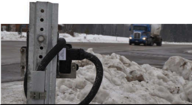
(Above) A rural intersection crash avoidance system in Wisconsin (Far left and below) The systems provide drivers (on both the major and minor roads) with a dynamic warning of other vehicles approaching the intersection
