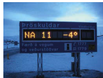
Variable message signs are used by Iceland’s ICERA to show windspeed, wind direction, temperature and, in extremely exposed areas, wind gust
